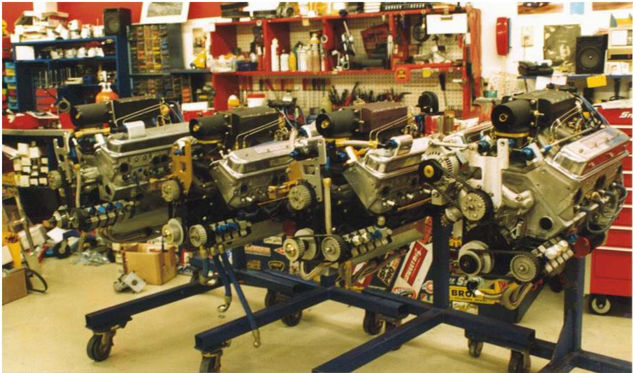
Small-block aircraft engines from 350 to 427 cu. in.
